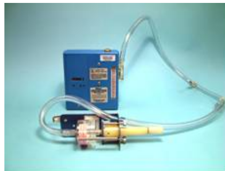
Pump with Bendix cyclone and filter
