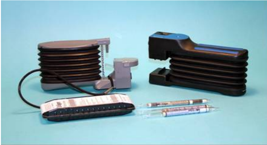
Drager Pumps with detector tubes
