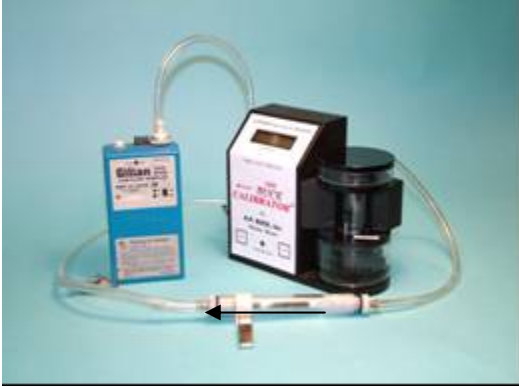
Calibration of a low flow pump with sorbent tube (Arrow indicates air flow)
