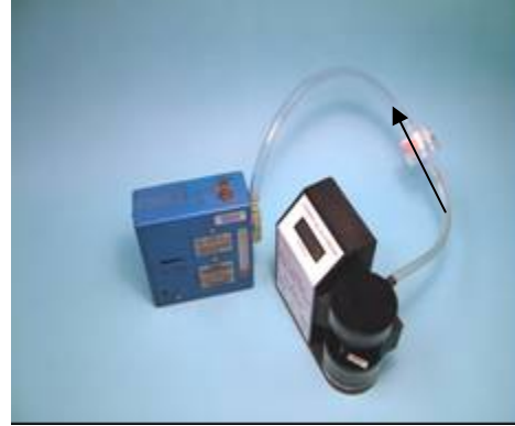
Calibration of a high flow pump with filter (Arrow indicates air flow)
