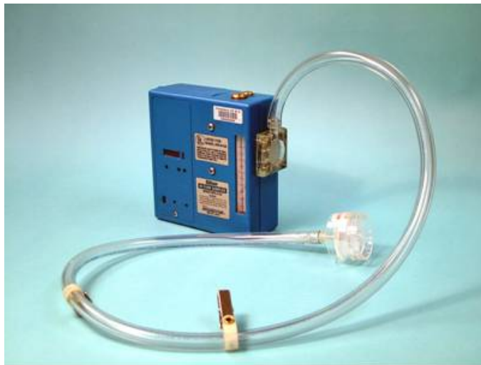
Pump with PVC filter
