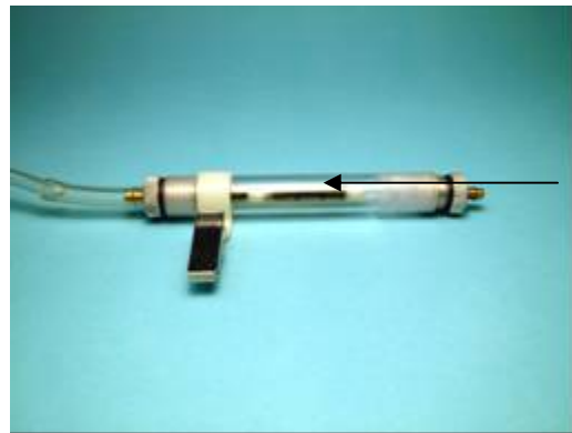
Sorbent tube in a holder. The large section of the media is to the right and the tube connects to the pump. (Arrow indicates air flow direction)
